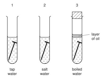
In which test-tubes do the nails rust?
